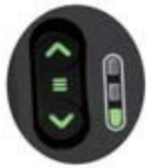
Figure 38: Drive function select button and display
